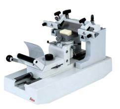
Designed for biomedical and industrial applications, the Leica SM2400 is a universal instrument for a variety of applications in all laboratories where paraffin or various industrial materials need to be sectioned. Its sturdy construction lends it qualities that ensure excellent sectioning results. The safety features of the system, such as a sledge locking device and knife guard are some of the outstanding features to guarantee convenient operation.
