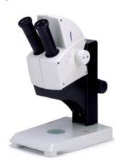
The Leica EZ4D, with its integrated 3megapixel CMOS camera and Leica application software, allows the direct storage of image data on 128 MB SD card or the connection to PC, Mac, video recorder or beamer. The application software included with the Leica EZ4D controls image capture and storage, live image display on connected PCs or Macs, and the archival and optimization of image data.
