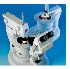
The modular design of the Leica EM CPC cryoworkstation facilitates quick and easy change of the cryofixation modules allowing plunge freezing of tissue into propane, bare grid method with ethane or metal mirror freezing (slam freezing) onto gold coated copper blocks.
