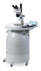
polymerization of resins. A stereomicroscope for viewing and positioning of the samples is available and the LED illumination from within the chamber makes work easy.
